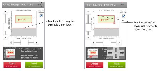
**NOTE:** If the acquisition times out (after 2 minutes), you can select **Back** to restart the adjust settings step or **Next** to accept the settings and continue to the next step. If acquisition times out, remove the tube and mix well before reloading and continuing.
